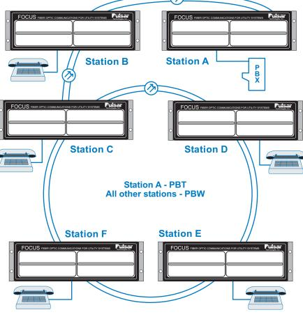
Other applications compatible with the PLE system include most automatic data collection systems and smart switches operating over dial-up modems. The benefits to you include reliable F.O. telephone channels over a single DS0 time slot.
