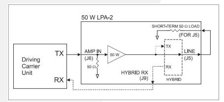
Typical connection diagram of one terminal of a PLC system with a 50 W LPA-2 inserted to boost the transmit power & the internal 50  $\Omega$  load temporarily connected to its Line Output for setting the TX power level. (Optional Hybrid shown in dotted lines.)
