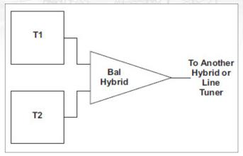
2. Skewed Hybrid for combining a TX/RX in a single FSK bidirectional channel
