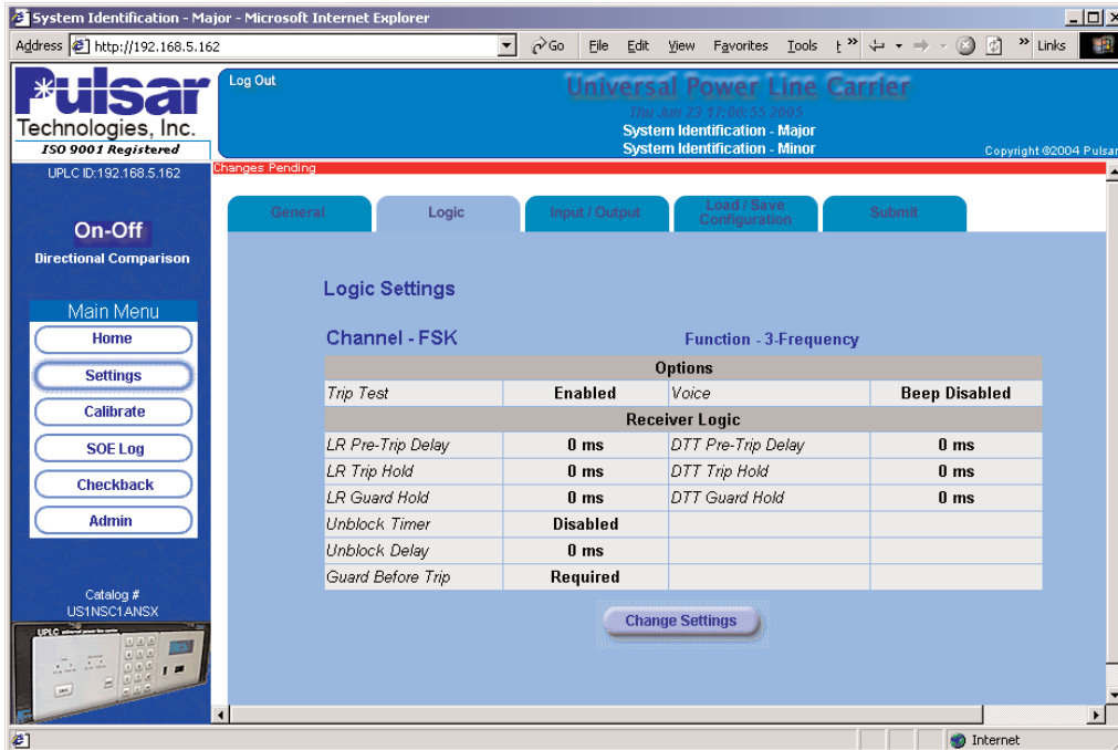
Figure 12. Example of The Logic Settings Tab for an FSK 3-Frequency Setting
