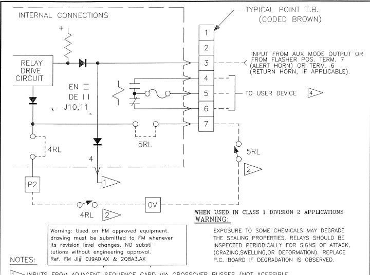
>INPUTS FROM ADJACENT SEQUENCE CARD VIA CROSSOVER BUSSES (NOT ACESSIBLE EXTERNALLY). SEQUENCE CARD MUST BE IN POSITION A (OR C) WITH 90AXC1 CARD IN POSITION B (OR D). SINGLE POINT SEQUENCE CARD MUST HAVE \*EL OUTPUT OPTION.
