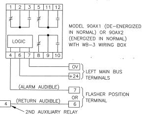
RELAY CONTACTS RATED 4 AMPS AT 250VAC OR 5 AMPS AT 28VDC OR 120VAC AND 0.5 AMP AT 125VDC RESISTIVE LOAD.
