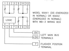
RELAY CONTACTS RATED 4 AMPS AT 250VAC OR 5 AMPS AT 28VDC OR 120VAC AND 0.5 AMP AT 125VDC RESISTIVE LOAD.
