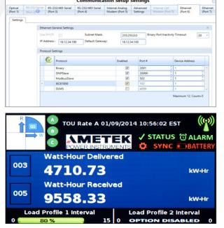
The color display makes it easy to view power measurements, phasor displays and meter diagnostics.
