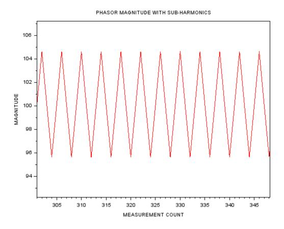
Fig.7: P class reference filter phasor magnitude in the presence of sub-harmonics
