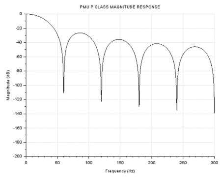
Fig.6: Magnitude response of the P class reference filter
