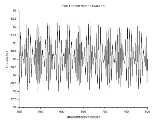
Fig.10: Frequency estimated by the P class reference filter during a simulated system disturbance
