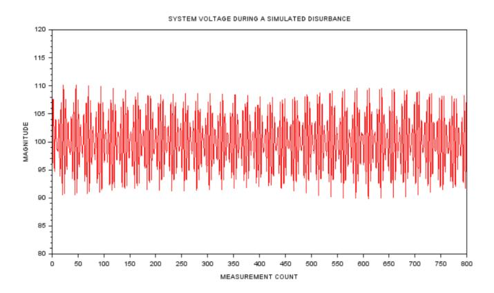
Fig.8: Phasor magnitude of the system voltage during a simulated disturbance
