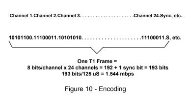
Once the incoming data is synchronized, it is separated back into 8-bit bytes, decoded into one of the 256 levels, and used to reassemble the waveform.
