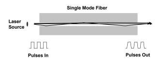
Fig. 7 - Dispersion for a Single Mode Fiber
