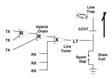
Figure 2 - Typical Power Line Carrier Terminal
