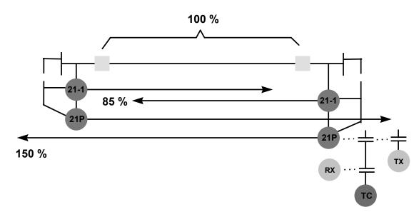
Figure 1 - Basic Distance Pilot Relay System
